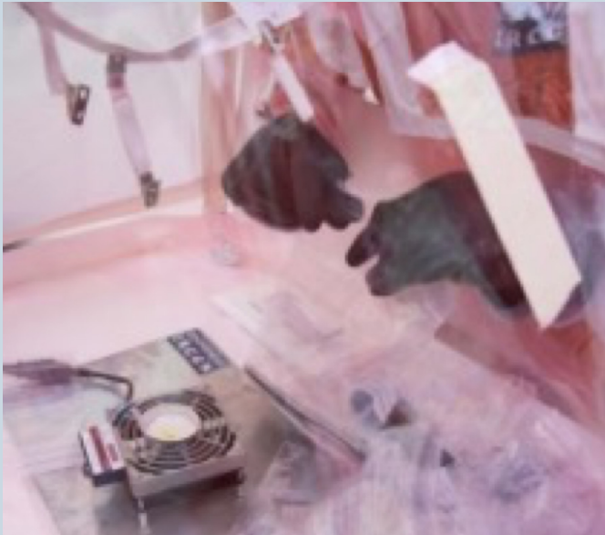
Figure 4. Cyanoacrylate fumigation tools placed in a glove/fume bag
