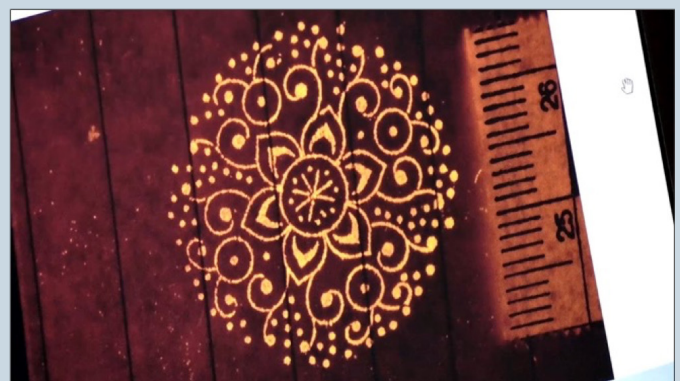
Figure 10. A 'fingerprint' photographed under monochromatic light, having been revealed by cyanoacrylate fumigation
