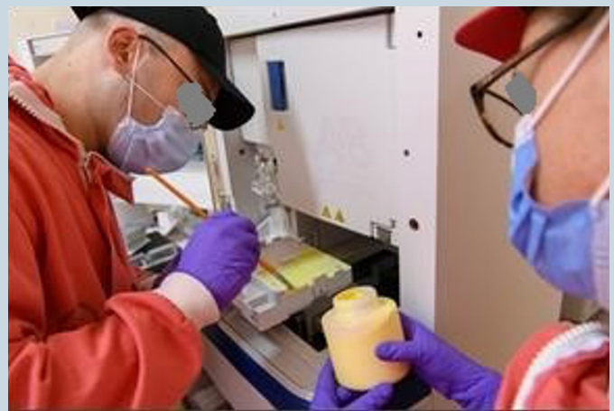
Figure 8. Protecting DNA sequencing device with decontamination gel
