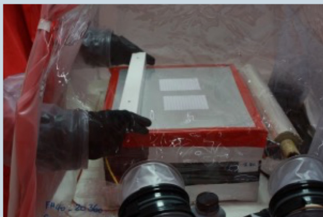
Figure 6. The use of an electrostatic toner powder to develop indented writing on pieces of paper in a vacuum box
