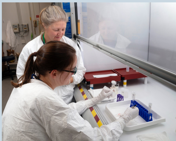
Figure 7. LLNL scientists dissolving an Epic Shadow sample for subsequent chemical purifications and measurements by mass spectrometry.
