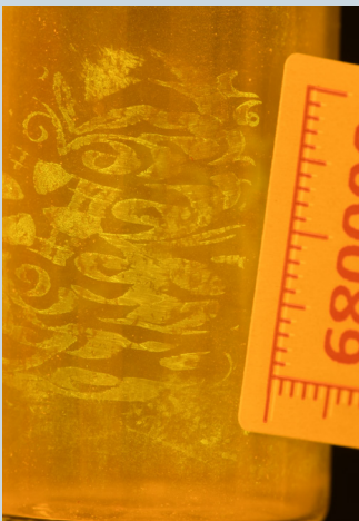
Figure 4. Areas of ridge detail enhanced with chemical staining and cyanoacrylate fuming located on 'Item 5/ ES-1'.
