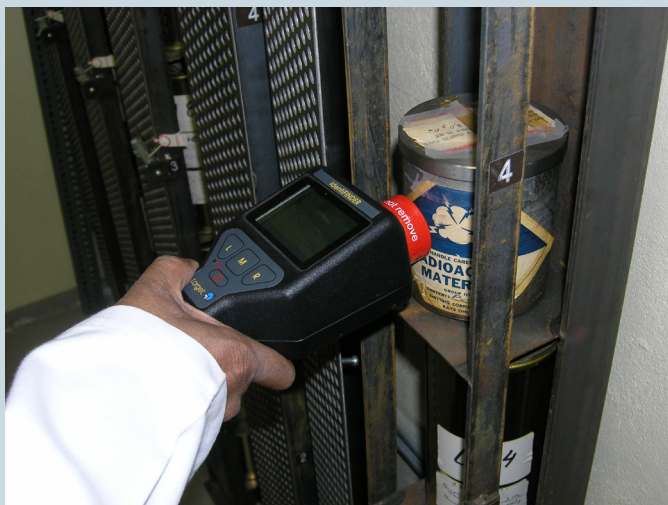
Figure 3. Measurements conducted at a facility in Norway using an IdentiFINDER
