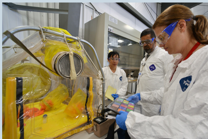
Figure 4. Nuclear forensic scientists performing an examination of the physical properties of nuclear or other radioactive material (pictured here in a glove bag) collected at a radiological crime scene
