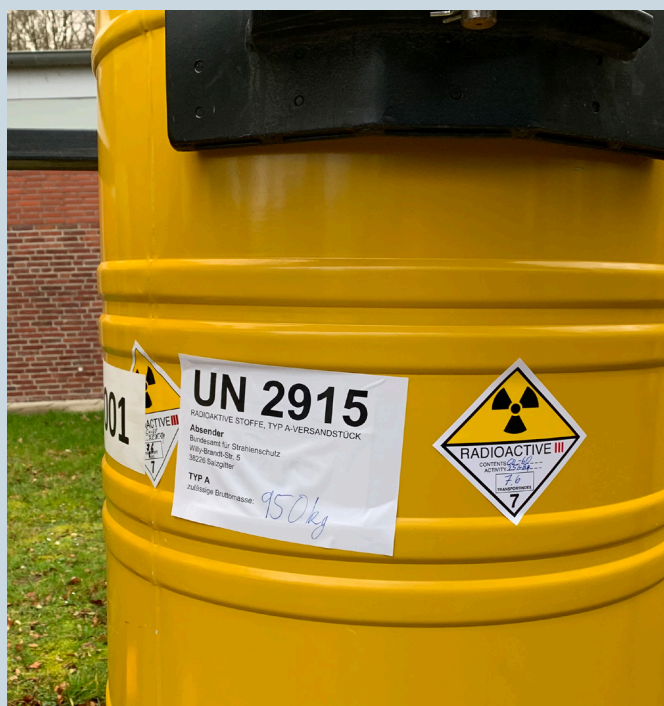
Figure 1. Type A package used to transport a Cobalt-60 source from a storage site to Radiochemistry Munich for further examination. The German Federal Office for Radiation Protection organized the transport in 2020.
