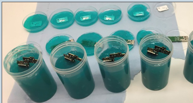
Figure 1. Decontamination of dismantled SIM cards, USB drives and iPhones with DeconGel 1120
