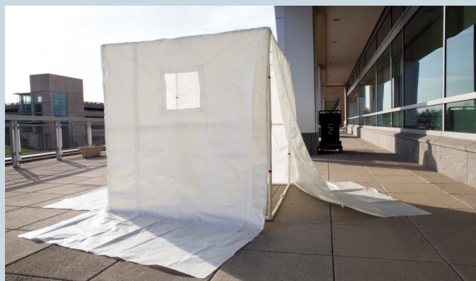
Figure 3. Encapsulating chamber built from kit components
