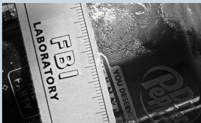
Figure 1. Example of a latent fingerprint developed using cyanoacrylate fuming
