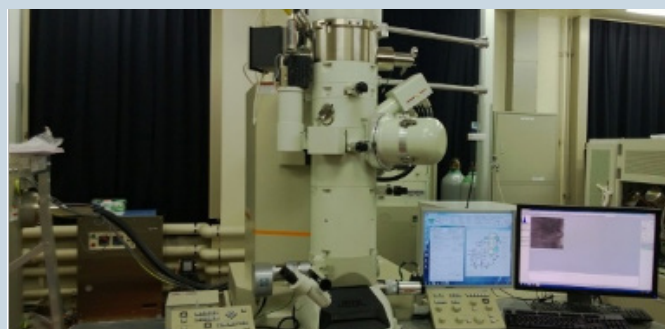
Figure 2. Transmission electron microscopy in the ISCN laboratory for Nuclear Forensics R&D
