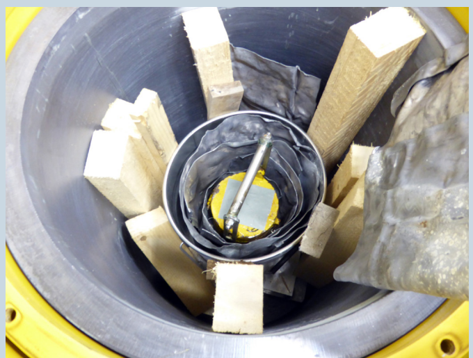
Figures 4 and 5. The use of the Type A container for shipping the Co-60 source found in Hamburg
