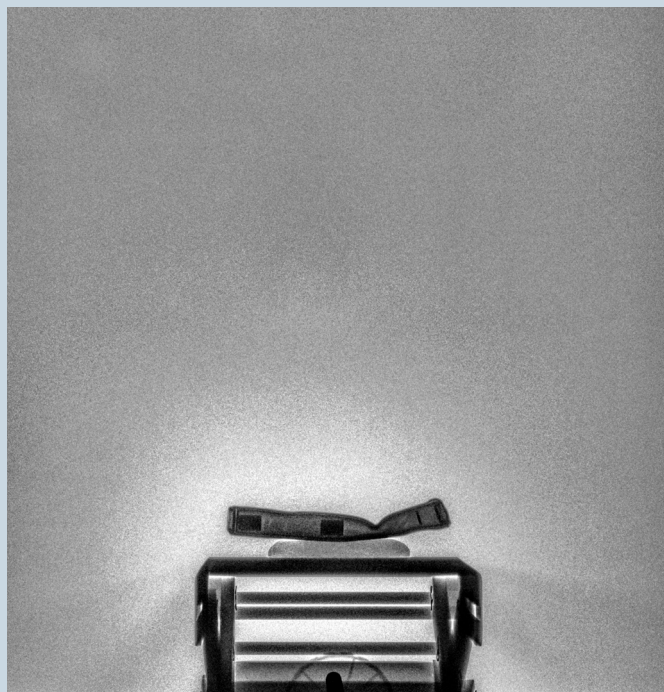
Figure 9. Autoradiography image of the Co-60 source discovered in Hamburg. Credit: BfS.
