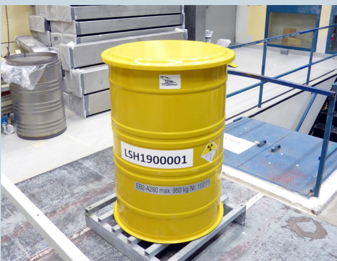
Figures 4 and 5. The use of the Type A container for shipping the Co-60 source found in Hamburg
